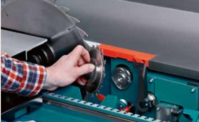
T6523 electrically adjustable 3-axis scoring saw
