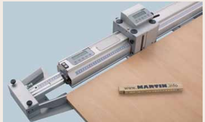
T6542 digital 2-point cross-cut fence
