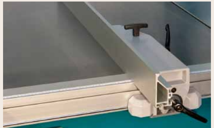
T6590 motorized positioning of the rip fence
