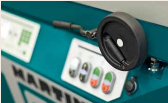
T6589 hand-wheel adjustment of the rip fence
